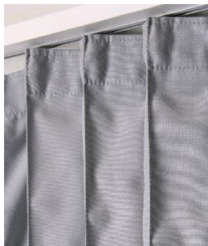
Appearance after washing 10 times at 40°C in a net bag and 3 times dry cleaning in a net bag
