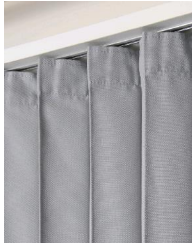
Appearance after washing 10 times at 40°C in a net bag and 3 times dry cleaning in a net bag
